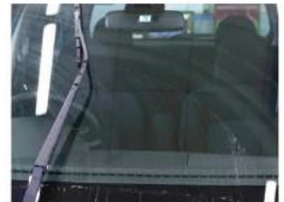
Unwiped parts due to deteriorated wipers
