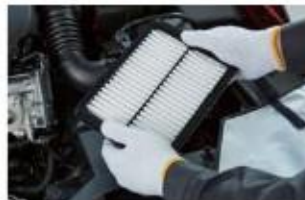
■ Air filter Contamination / clogging / damage
